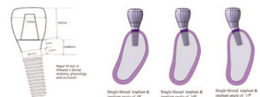
• Fig. 2. (Left) Design a dimension of restored prosthesis that cervical-occlusal is 8,5 mm and buccolingual is 7,5 mm according to Wheeler's dental anatomy, physiology and occlusion. (Right) Schematic drawing of the different implant angulation that is 0°, 10° and 15° in a bone.
